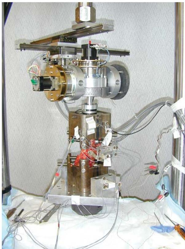
Figure 2. The test setup in the six-degree-of-freedom spinal simulator.
