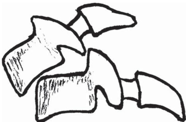
Figure 1. Schematic drawing of the distractive–flexion stage 3 injury, DF-3. The upper vertebra is dislocated in flexion in relation to the lower one. Both facet joints are dislocated, but the overall anterior displacement is less than 50%. An observation from the creation of the injury in the specimen was that the posterior longitudinal ligament had to be torn in order to allow dislocation of the joints.
