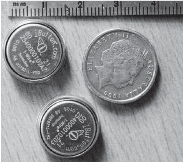
Figure 1. The Thermocron (Maxim Integrated Products, Inc., Sunnyvale, CA, USA) is 15 mm in diameter and is equipped with a temperature sensor, memory, and battery.
