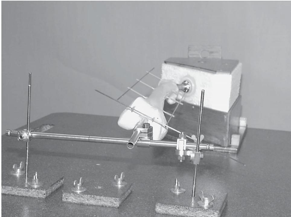
Figure 2. Simulation of flexion, abduction and rotation. The angles of the guide wires in relation to the board were measured with a goniometer. Each position was fixed with screws when taking a radiograph.
