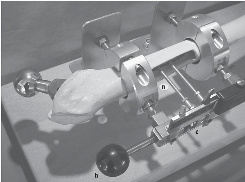
Figure 3. The femoral component was fixed with two screws (a) on the measuring frame and could be moved along the axis of the femur. Subsidence was simulated by turning the handlebar (b) and measured with the slide calliper (c).
