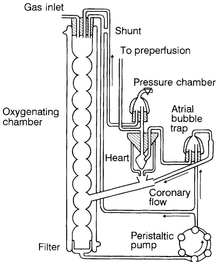
**Fig. 3. Perfusion apparatus for isolated working rat heart.** See text for description.
