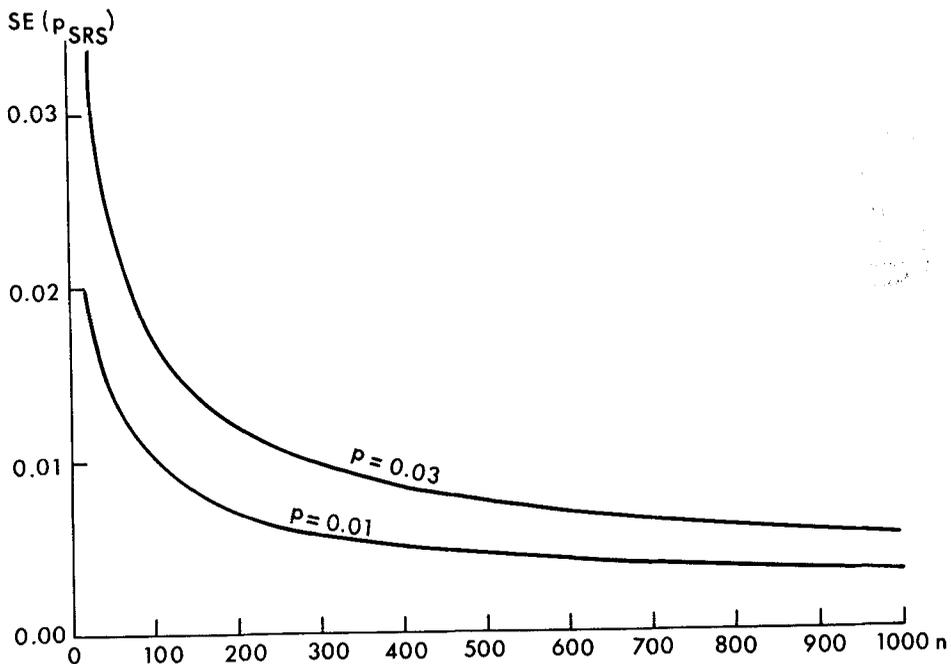
Figure 1 - The standard error of  $p_{SRS}$  as a function of the number of observations,  $n$ .
