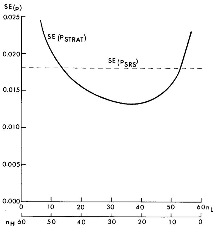
Figure 2 - The standard error of  $p_{\text{strat}}$  for different sizes of  $n_L$  and  $n_H$  with  $P=0.02$  and  $n_L + n_H = 60$ .
