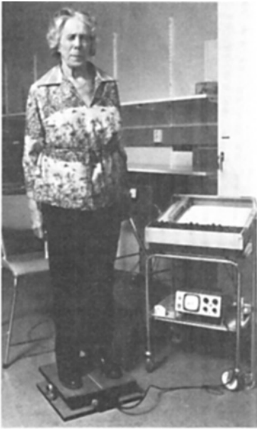
Fig. 3. Stroke patient (left hemiplegia) standing on a force platform for balance tests by methods described by Eklund and Löfstedt (5). Photograph: Leif Kumlin, University Hospital, Uppsala.
