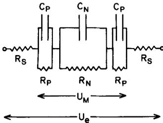
Fig. 1. Equivalent circuit of a membrane showing the external solution resistances ( $R_S$ ), the electrical parameters of the surfaces ( $R_P$ ,  $C_P$ ) and of the nonpolar region ( $R_N$ ,  $C_N$ ).  $U_M$  is the potential difference across the membrane and  $U_e$  is the total potential difference between the electrodes.
