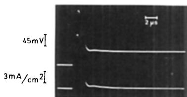
Fig. 2a. Potential (upper) and current (lower) records from a voltage clamp experiment with 0.1 M KCl,  $10^{-6}$  M monoactin-dinactin mixture and 2% PE.
