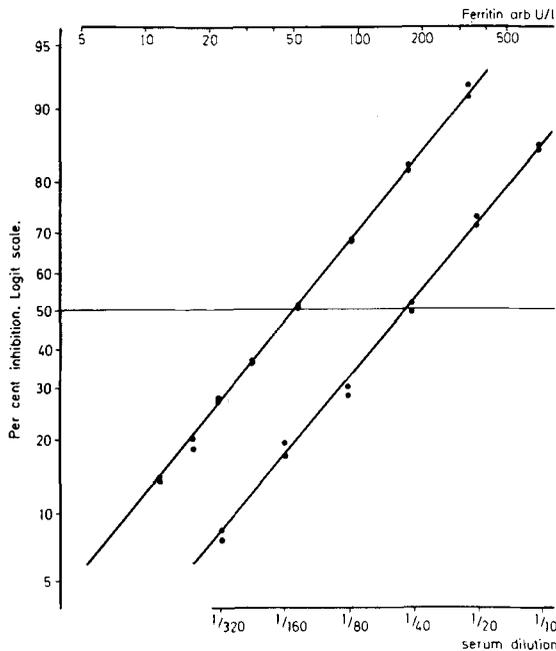
Fig. 1. Logit representation of the dilution curve for the reference standard and for serum sample with high ferritin content.
