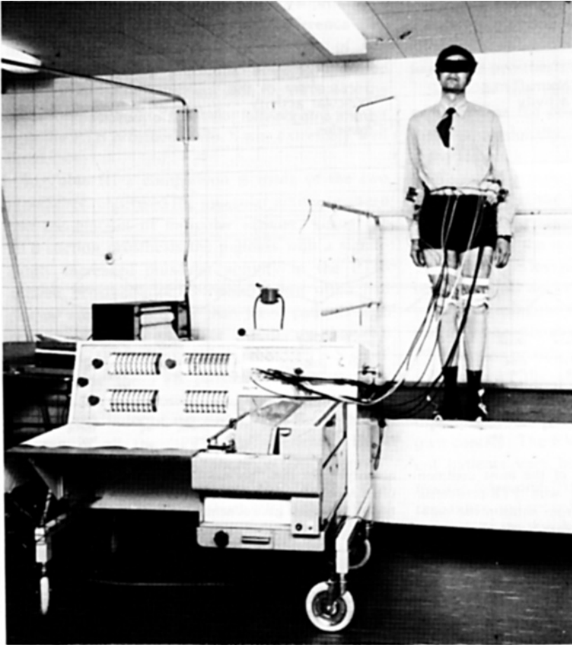
Fig. 2. The electromyographic recorder, a modified Elema-Schönander EEG-apparatus.
