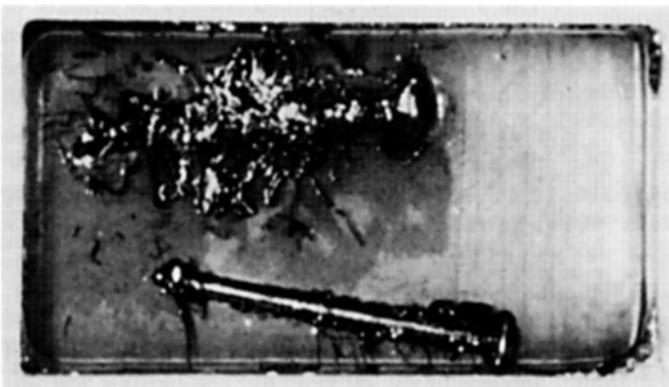
*Fig. 6.* Galvanized nail with a distinct, strong reaction after 15 seconds in the ferroxyl gel.
