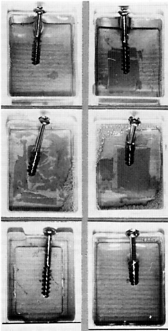
Fig. 4. Ferroxyl test on removed A0 screws after implantation times of up to 36 weeks. No corrosion was found.
