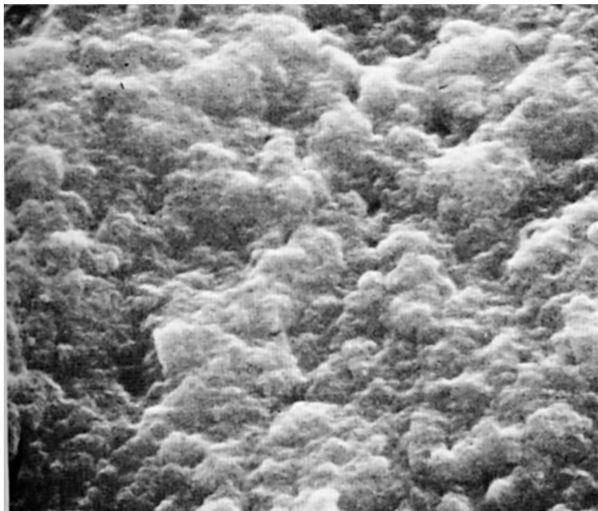
*Fig. 1.* Membrane fraction, prepared without the colloidal solution of silica.  $\times 2000$ .
