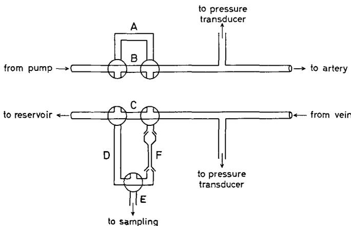
Fig. 1 b. The injection and sampling device. Upper catheter is "arterial". Blood goes via either route A (injection) or route B. Below the "venous" catheter is shown; Route C, free flow; Route C-D-E, sampling in free flow. Route F includes a thin exchangeable catheter producing venous congestion with or without sampling.
